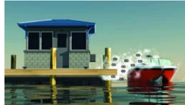
Exhausts traveling along obstruction.
