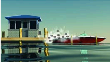
Blockage of boat exhausts by obstruction.
